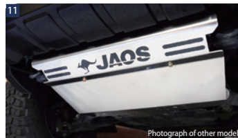
11 JAOS SKID PLATE TYPE R ■ 4.0mm thick A5052 ■ Include: JAOS logo sticker
