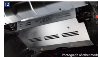
12 JAOS SKID PLATE 3 ■ Shot blasted 2.5mm thick SUS304
