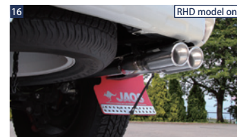
BATTLEZ TAILPIPE FINISHER TF-2 ■ SUS304 ■ Mine pipe : 60.5φ Finisher : 115×61(4pcs.)
