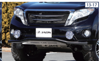
09 JAOS FRONT SKID BAR ■ Black powder coated or Polish 60mm SUS304 tube, Black powder coated or Shot blasted 2.5mm thick SUS304
