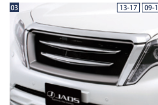
03 JAOS CHROME BLADE GRILLE ■ Flame : Unpainted FRP, Chrome ABS garnish
